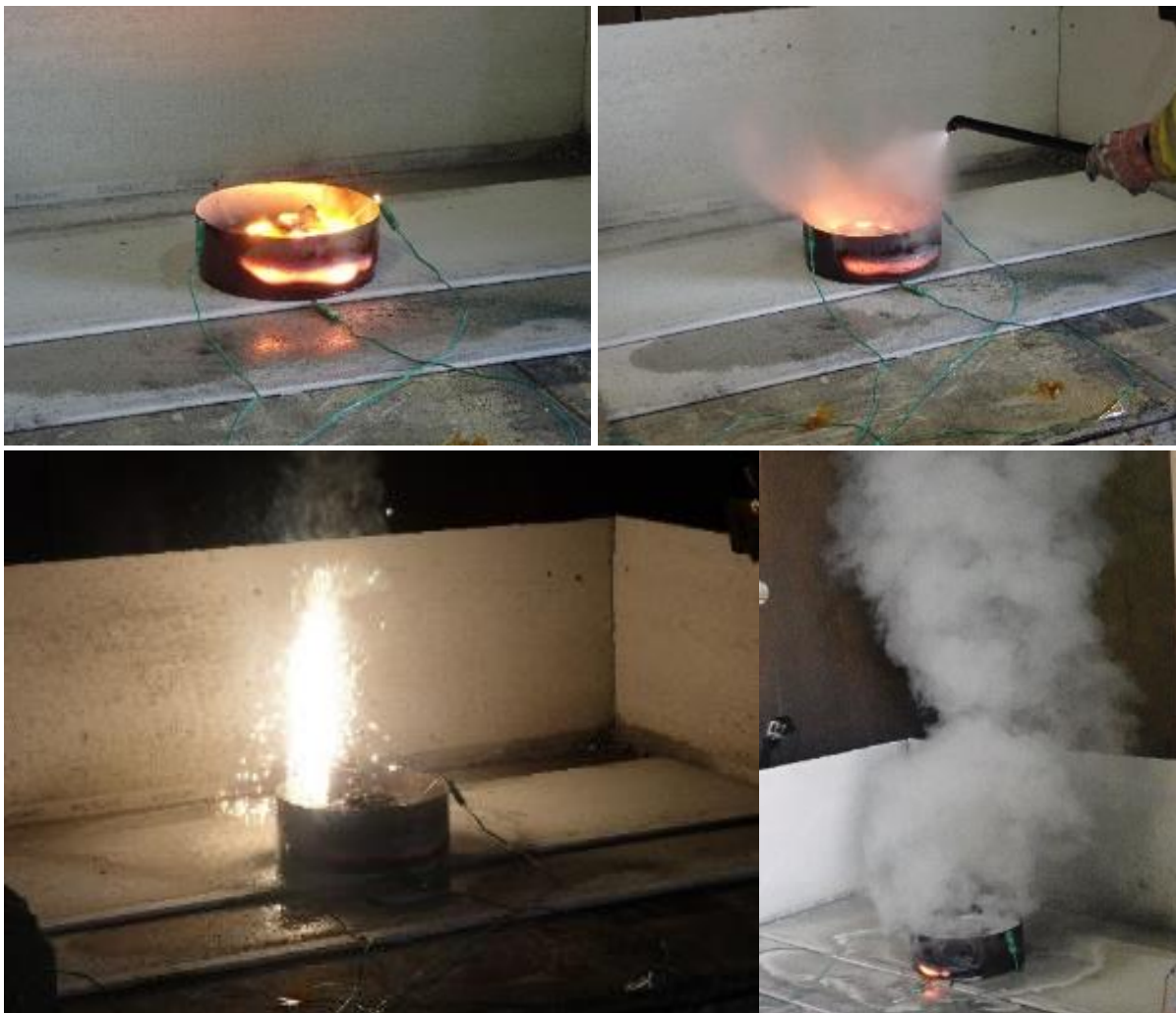
Figure A3-13 The response of titanium dust in a drum after application of F-500
