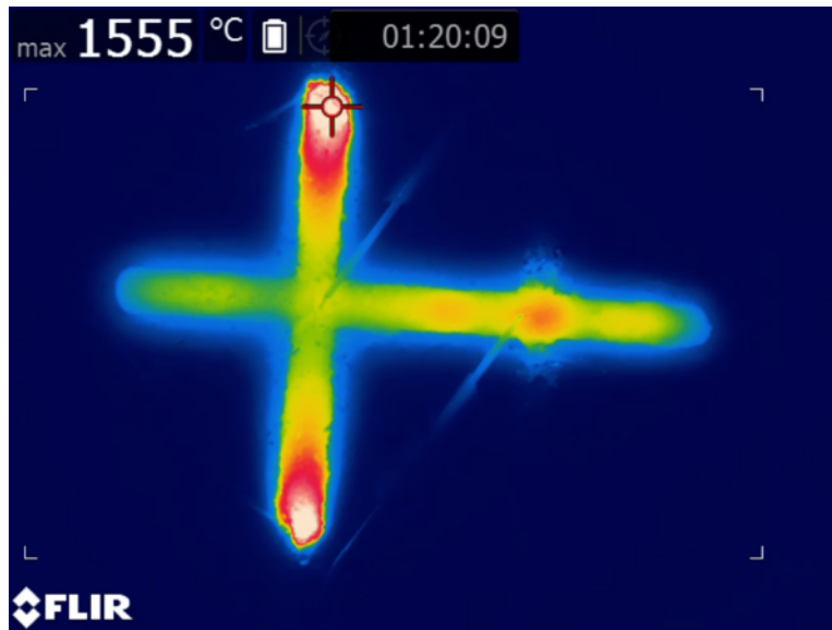
Figure A2-19 Thermal image of the double cross trough of test shown in Figure A2-18
