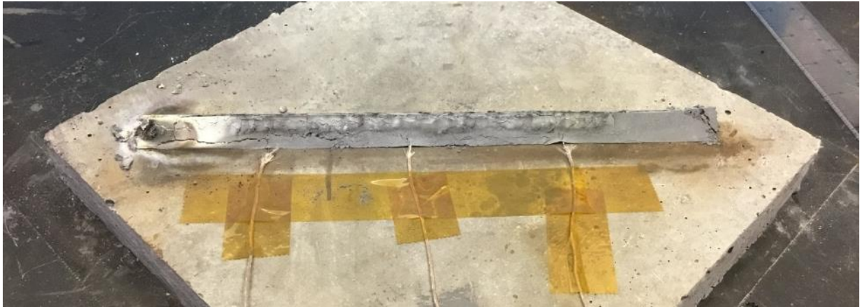
Figure A2-24 Smoldering combustion along prismatic train of zinc-rich baghouse dust
